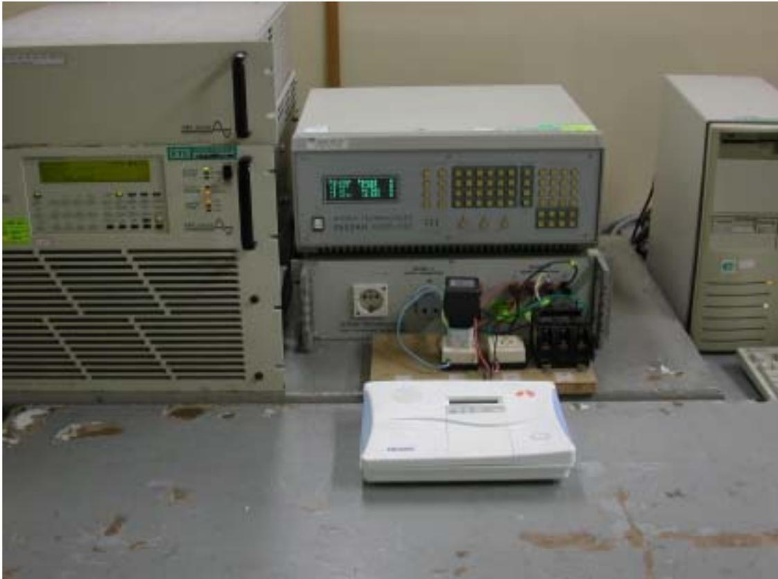
**4. Electrostatic Discharge Immunity Test Setup Photo**
